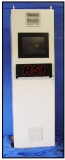
A typical upgrade requires only the installation of a new Main Electronic Cabinet (MEC) and an optional remote operator panel.
